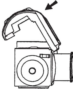
2. Install the mouth piece (10) and the locking strap (9). Tighten and cut off locking strap with plastic band pliers.
