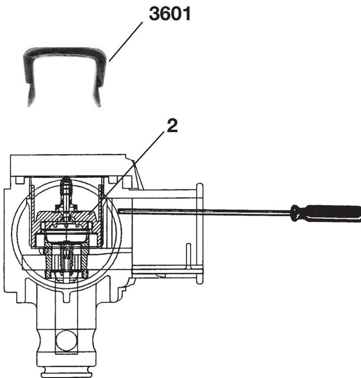
1. Press down the removal tool carefully so that the holders bend inwards and the servo valve "pops up".
