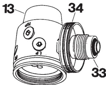
2. Fit the connection (33) to the wheel (34) and screw it into the valve housing (13) with a 6 mm Allen wrench. Place the valve housing in torque wrench to 28 - 30 Nm. (20-22 lbf.ft).
