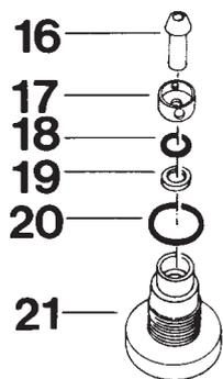
3. Remove the valve piston (16) and the spacing sleeve (17). Remove the o-ring (18) with an o-ring remover. Remove the washer (19) and the o-ring (20). Use an o-ring remover for this also. Make sure the sealing surfaces are not damaged.
