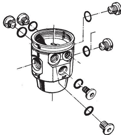
2. Screw in the blind screws in the LP- HP outlets. Use a 5 mm Allen wrench and tighten up by hand.
