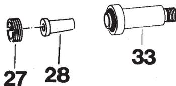
3. Install the cup filter (28) screw in the locking screw (27) with an 8.5 mm screwdriver.
