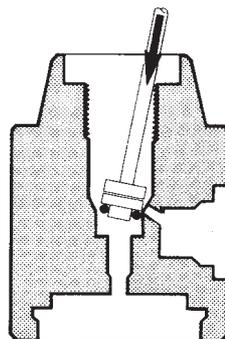
3. Install the o-ring (14) on the valve seat (15) and the install the valve seat with a seat drift. Press the drift diagonally as shown in the diagram and the "rock" it to the vertical while pressing down. The seat and o-ring should pop into place. This procedure avoids damage to the o-ring from the high pressure supply outlet.
