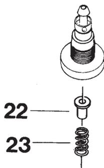
2. Remove the spring (23) and the spring guidance (22).
