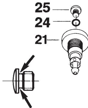
1. Steady the balance housing with a special wrench. Then remove the blind screw (25) with a 5 mm Allen wrench. Remove the o-ring (24) with an o-ring remover. Remove the balance housing (21) with the special wrench.
