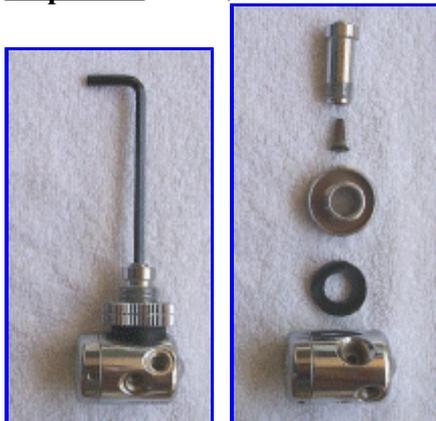
Parts (top to bottom, right photo): DIN stem, filter with O-ring, threaded DIN connector, distance piece, regulator housing
