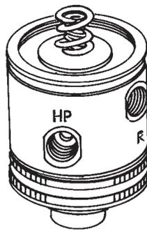
2. The inner and outer secondary springs shall be set in the middle.
