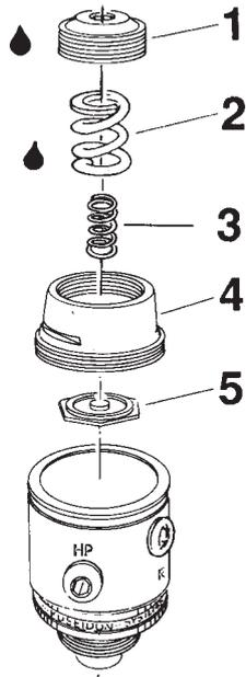
1. Place the upper diaphragm center (5) on the diaphragm in the valve housing.
