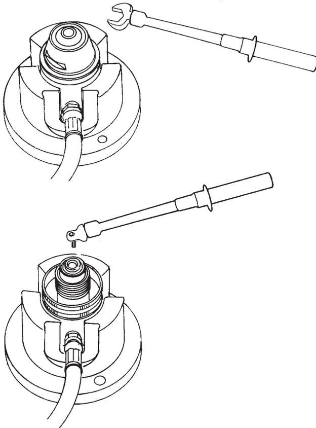
Place the stage assembly in the fixture. Tighten the valve housing cover with a 27 mm crowsfoot and the connection with a 6 mm Allen wrench. use a torque wrench to achieve 28-30 Nrn (20-22 lbf.ft) of torsion.
